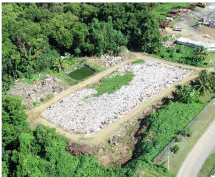
Entire view of the current final disposal site of Kosrae taken by a drone. The ventilation pipes in the middle of the disposal area and the leachate pond annexed are seen in the picture.
