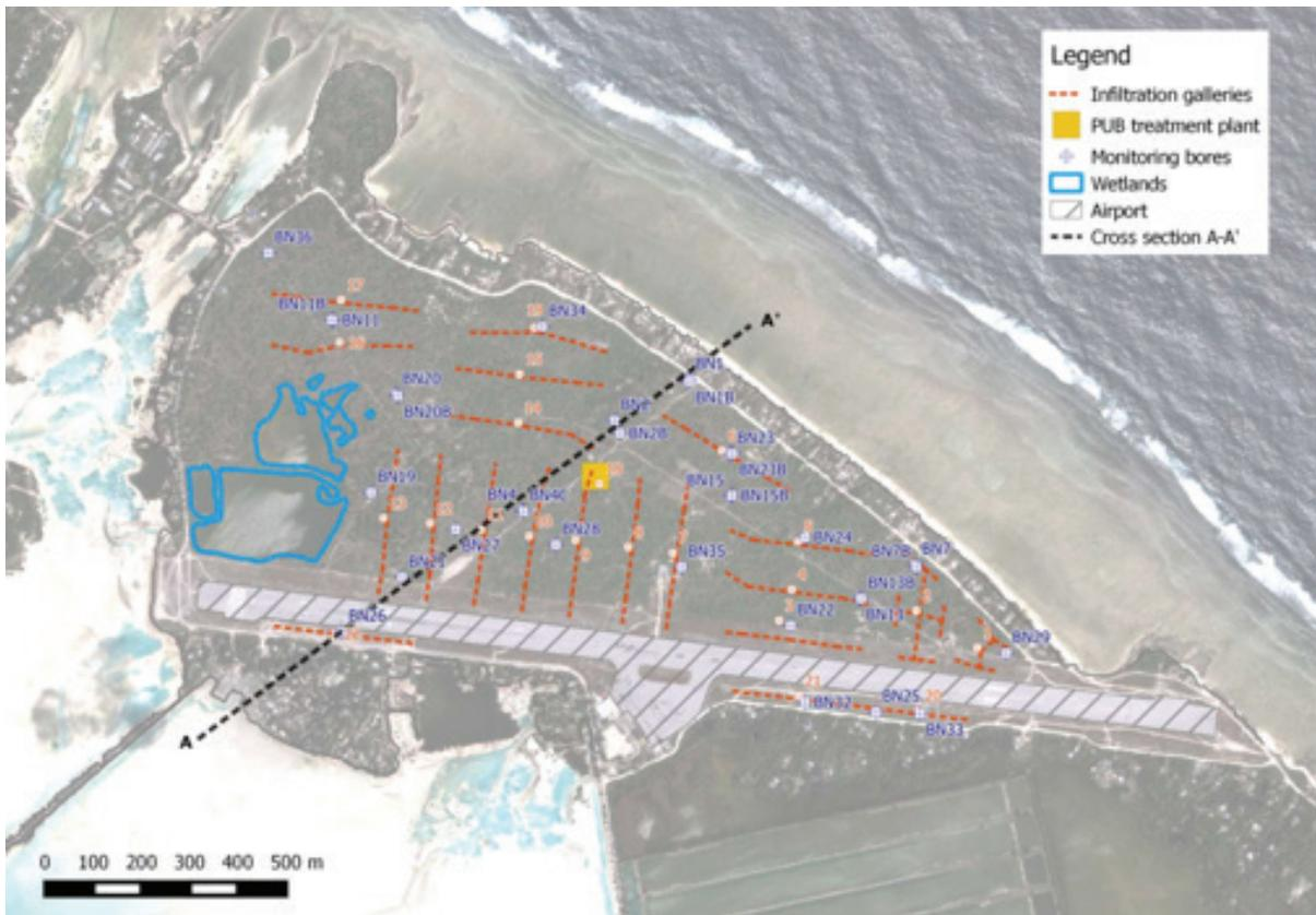
Figure 2. Depicting the Bonriki water reserve infiltration galleries, monitoring bores, wetlands, etc. (adapted from Galvis-Rodriguez, S et al. 2017)
