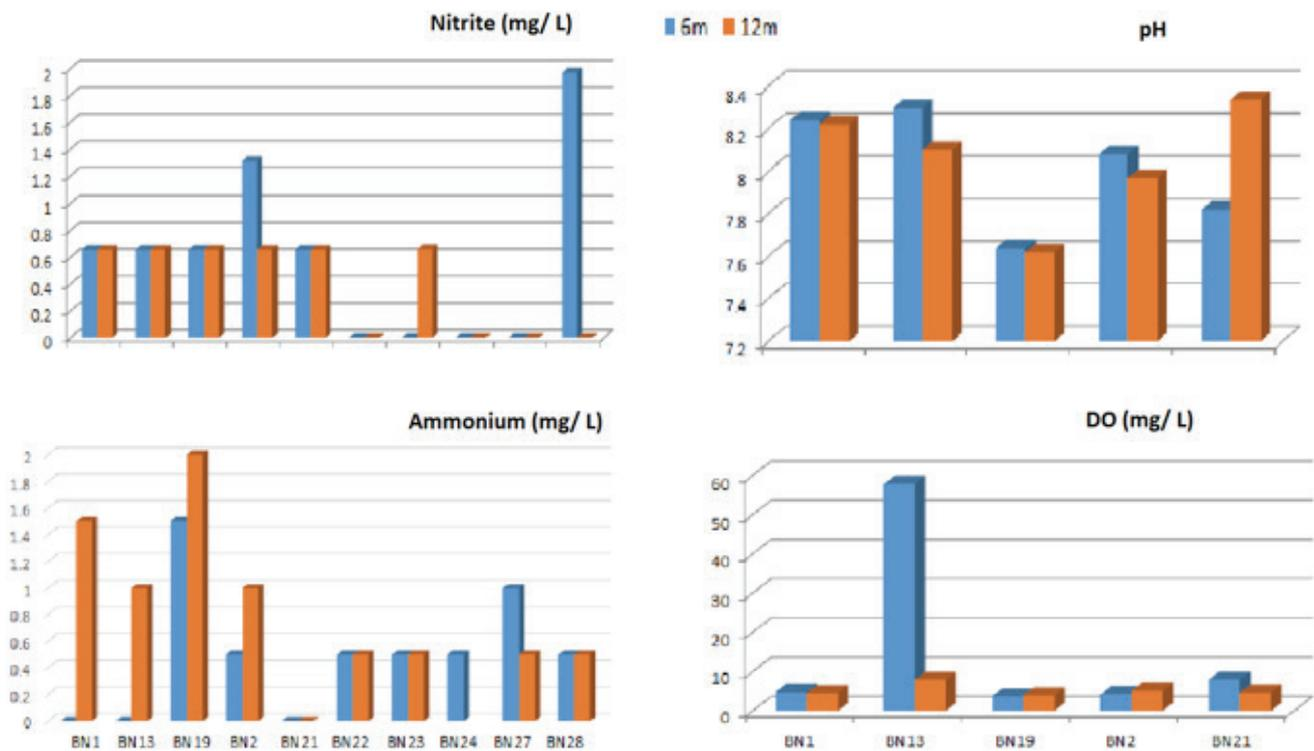
Figure 7. Comparing several water quality parameters between 6m and 12m depth.
