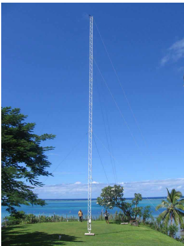
One of 16 meteorological stations established by the Fiji Dept of Energy to monitor for appropriate wind energy sites. Source, Ministry of FA, 2013.
