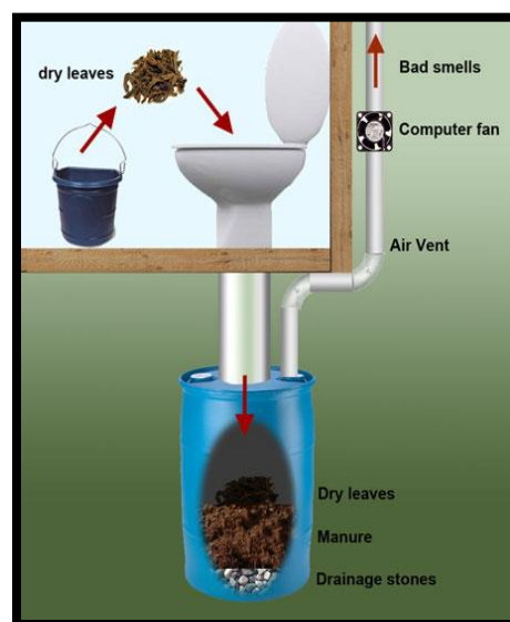
Fig 18: How compost toilet works Source: http://www.ecofilms.com.au/tanias-compost-toilet-tour/
