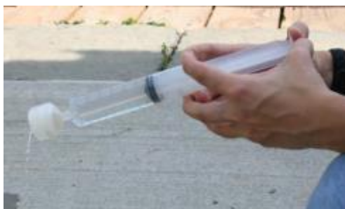
Figure 10: Pushing water through the syringe filter for chlorophyll a sampling
