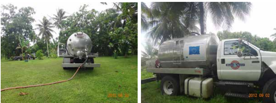
Figure 15: The Majuro Water and Sewer Company septic pump-out operations
